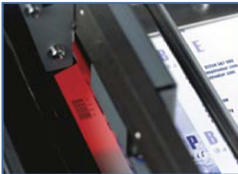
Figure 53: Barcode reader automatically sets up pre-programmed jobs
