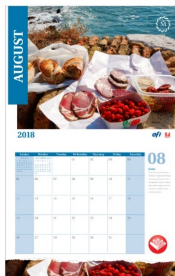
Calendars using gangup-repeat imposition style and top binding edge
