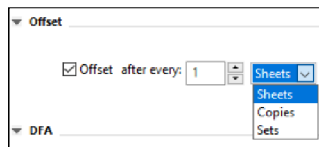
Offset setting in the Job Properties' Finishing tab.
