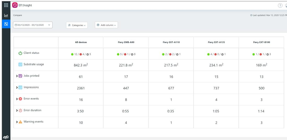
The screenshot shows the EFI Insight interface with a comparison table for the period 03/13/2020 - 03/13/2020. The table compares 'All devices' with four specific Fiery device models: Fiery EMB-A80, Fiery EXT-A110, Fiery EXT-A135, and Fiery EXT-B100. Metrics include Client status (with status indicators), Substrate usage (m²), Jobs printed, Impressions, Error events, Error duration, and Warning events.
