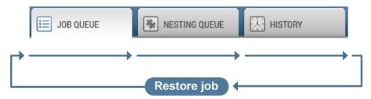
The workflow steps are as the arrows above show from left to right. Files are imported into the system in the Job Queue, then processed through the Nesting Queue, then finished and saved into History Queue. Files can easily be Restored again from the History Queue into the Job Queue.
