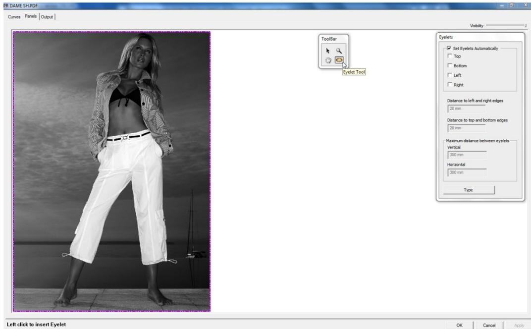
Select the **Eyelet tool** in the Panel Tool bar to get the Eyelet Dialog for specification of the eyelets.
