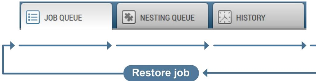
The workflow steps are as the arrows above show from left to right. Files are imported into the system in the Job Queue, then processed through the Nesting Queue, then finished and saved into History Queue. Files can easily be Restored again from the History Queue into the Job Queue.
