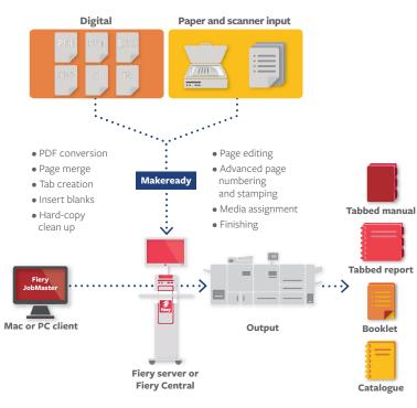
Flexible architecture allows you to perform makeready tasks from a client or locally at the Fiery or Fiery Central server.
