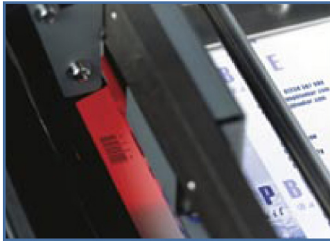
Barcode reader automatically sets up pre-programmed jobs
