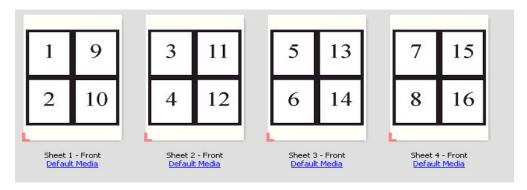
The Duplo — Long Edge Feed Imposition Layout orders pages sheet wise in line with columns or rows perpendicular to the longest sheet edge, optimizing page layout to fill the rows and columns on a sheet.
