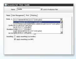
Agfa Apogee queries Fiery controller through JDF/ JMF for the media in Fiery Paper Catalog. Apogee operator can select the right media directly from the Apogee UI.
