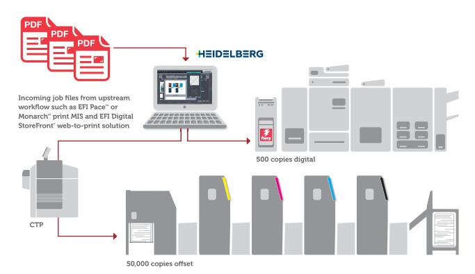
Heidelberg Prinect integration with EFI™ Fiery® digital print servers creates a single workflow management system for offset and digital printing. The hybrid workflow provides a significant impact on efficiency in many production scenarios: long or short job run lengths, a mix of static and variable components, or creating quick proofing with digital press for longer offset press runs. Each job can be routed
