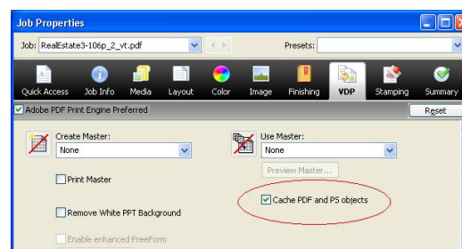
“Cache PDF and PS objects” box in the VDP tab of Job Properties
